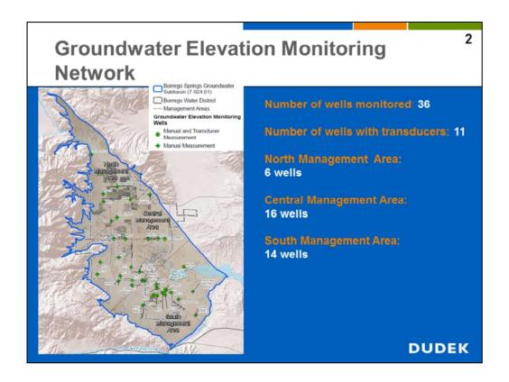
The Borrego Valley Groundwater Sustainability Agency (GSA) groundwater elevation monitoring network currently consists of 36 wells in the Borrego Springs Subbasin. An additional 4 wells are monitored for groundwater levels in the Ocotillo Wells Subbasin. This presentation is focused on the results of the Borrego Springs Subbasin (Subbasin).
