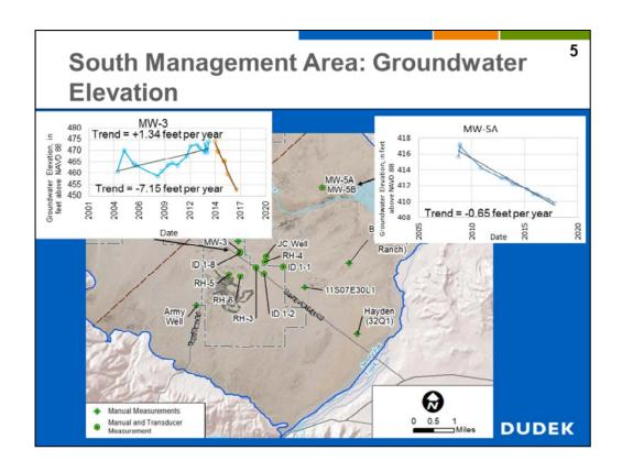
Well MW-5A located in the Borrego Sink in the SMA indicates a declining groundwater trend of 0.65 feet per year. This well is located far from large pumping centers.
