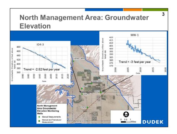
Historical groundwater levels in wells ID4-3 and MW-1 indicate a declining trend of 2.5 to 3 feet per year in the NMA. Each well hydrograph has a distinct period of record and number of data points based on when the well was originally drilled, lifespan of the well and frequency of data collection.
