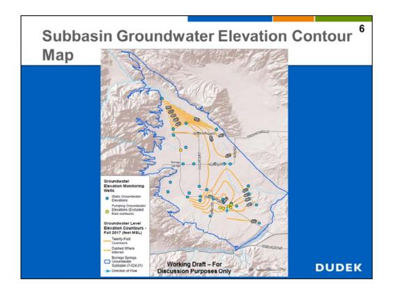
Groundwater elevation contours shown in the figure represent groundwater elevations measured in the fall of 2017. Groundwater elevations decrease from the north end (at Coyote Creek), and south end (near Rams Hill) of the Subbasin towards the center of the Subbasin near the town of Borrego Springs, where the current groundwater elevation is approximately 400 feet above the NAVD 88 datum.
